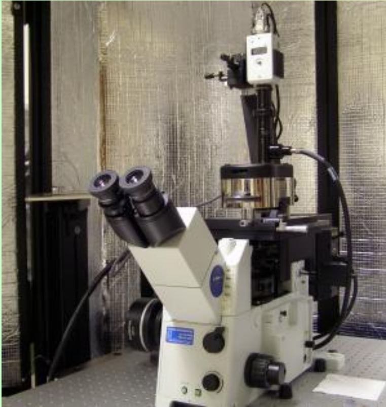
MFP-3D AFM Microscope from Asylum Research mounted on Inverted Optical Microscope from Olympus.
