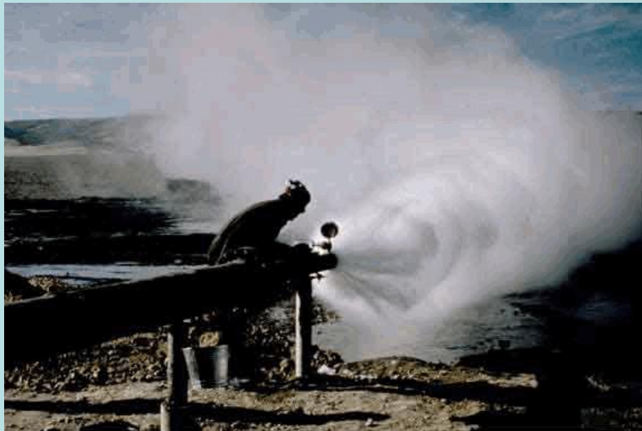
If a reservoir is discovered, characteristics of the well and the reservoir are tested by flowing the well.
