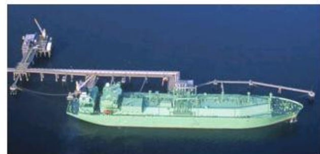
LNG is transported in large ships that are fitted with a special cargo containment system inside the inner hull to maintain the LNG at atmospheric pressure and minus 260 degrees Fahrenheit. (Click for an expanded view.)
