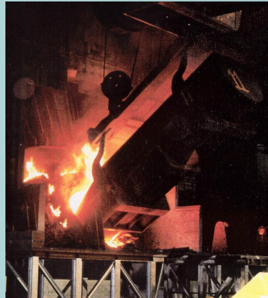
Scrap charging in a converter shop
