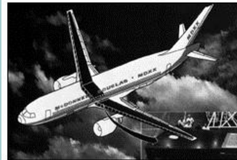
Here, the full span of the stitched/RFI wings is shown. Composites will make up all but the leading and trailing edges of the wing. The largest portion of the wing, called the wing stub-box (shown bottom right), was tested at NASA Langley in July, 1995.
